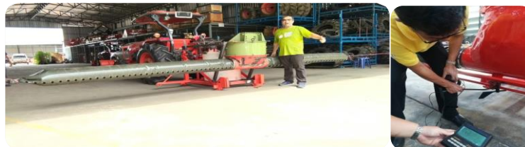
Figure 4 Air flow measurement test in laboratory
