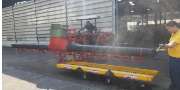
Figure 2 Spraying coverage zone and distance test of nozzle
