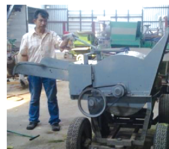
Figure 9 Fiber plant chipping machine
