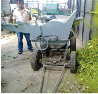
Figure 10 chipping oil palm branch, Figure 11 Mixed chipping plant with Salaka branch, Pineapple waste, Empty oil palm fruit Bunch
