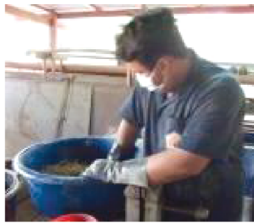
Figure 11 Mixed chipping plant with cement
