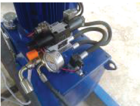
Figure 37 electrical valve and Relief valve
