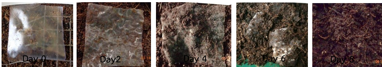
Figure 18. Photo of cassava starch films with plasticizer of biodegradation studies in soil burial on 0, 2, 4, 6 and 8 days.
