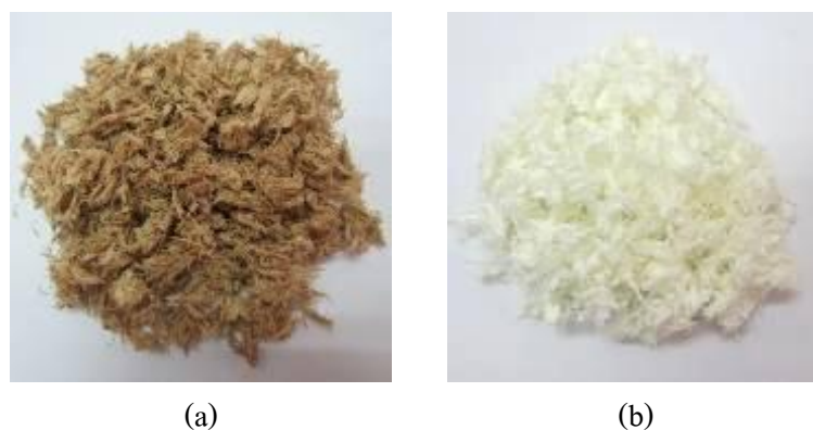
Figure 17 Illustrates the cellulose from durian husk. (a) Cellulose was extracted with 1 M NaOH at 80-90 °C for 1 hour. (b) Cellulose after bleaching with 30% H 2 O 2 at 80-90 °C for 20 min.
