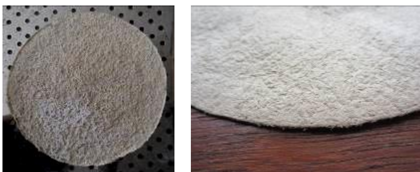
Figure 8 Illustrates the preform after dried at 55 °C
