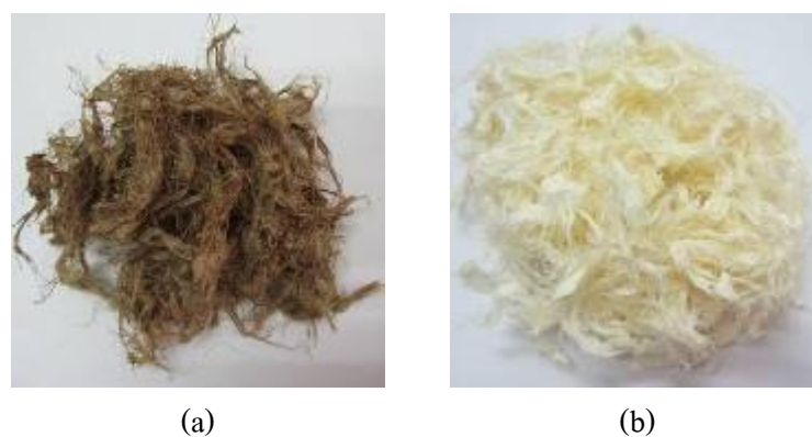
Figure 18 Illustrates the cellulose from banana pseudo-stem. (a) Cellulose was extracted with 1 molar NaOH at 80-90 °C for 1 hour and (b) cellulose after bleaching with 30% H 2 O 2 at 80-90 °C for 20 min.
