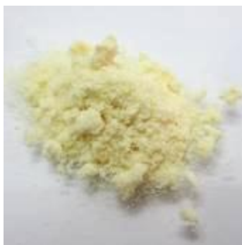
Figure 49 Carboxymethyl cellulose (CMC) powder, which synthesized by reacting alkali-cellulose with chloroacetic acid, yield = 138.12%, purity = 95.63%, color score: L^* = 85.82 a^* = -0.67 and b^* = 18.05
