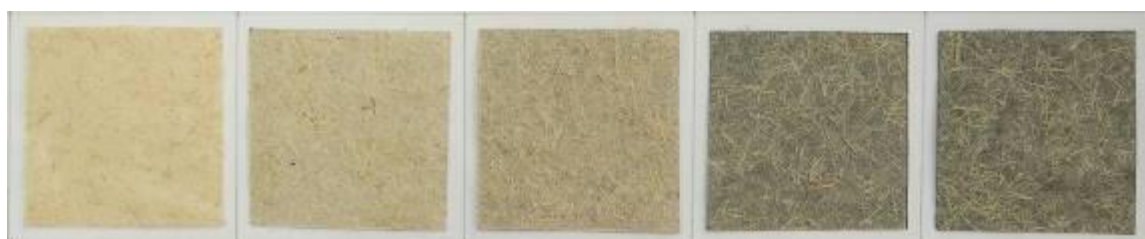
Figure 27 Ethylene absorber paper with various activated carbon powder content; left to right 0, 5, 15, 25 and 35% w/w
