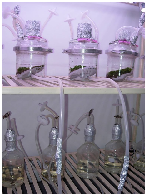
ระบบ Disposable system Glass system (using air pressure pump)
