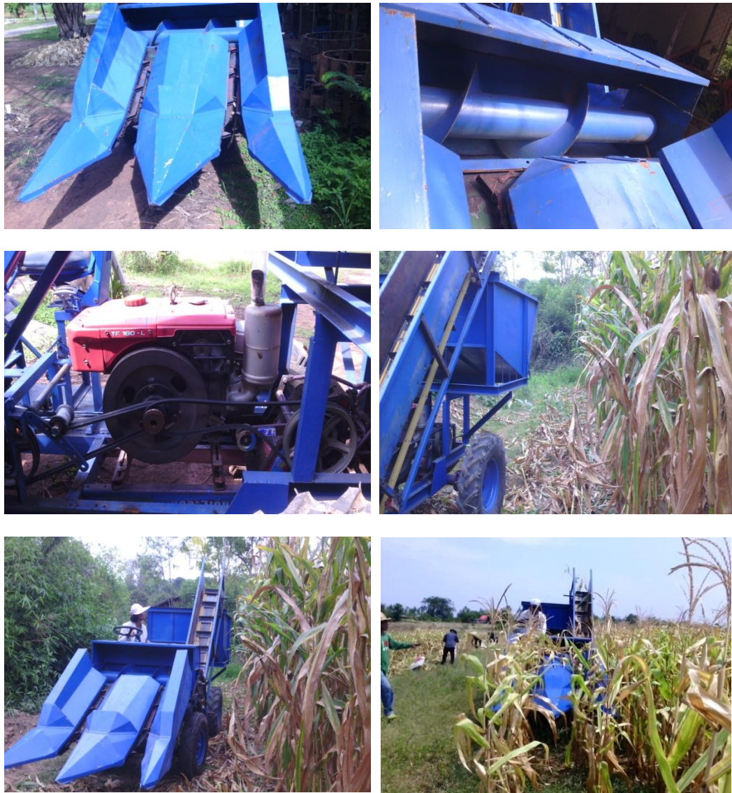
Fig.1 Maize Snapper two rows type
