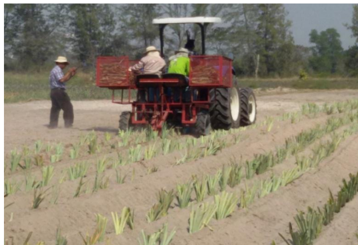
Figure 8 Pineapple transplanter attached with tractor 50 Hp
