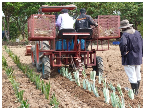
Figure 6 Pineapple transplanter attached with tractor 45 Hp
