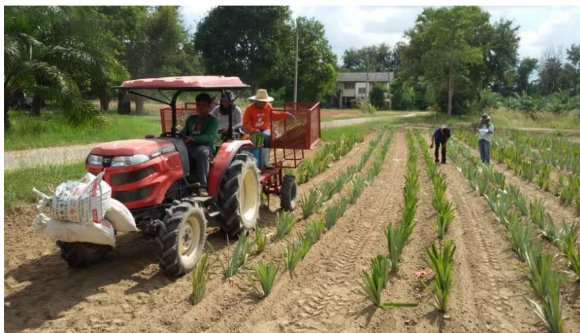
Figure 7 Pineapple transplanter attached with tractor 39 Hp
