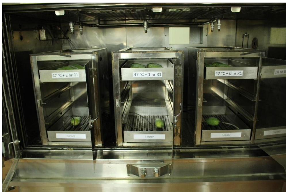
Figure 2 Injury test of Modified vapor heat treatment (MVHT) on Ok Rong mangoes using Sanshu Vapor Heat Treatment System (Differential Pressure Type model EHK-1000D)
