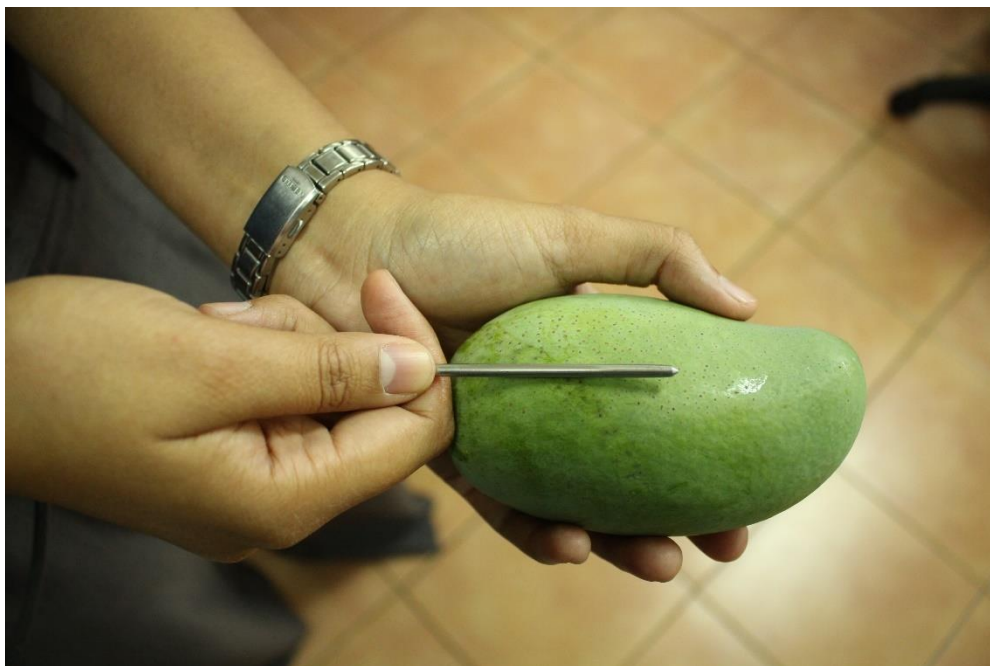
Figure 3 Fresh Ok Rong mango fruit with a fruit thermal sensor
