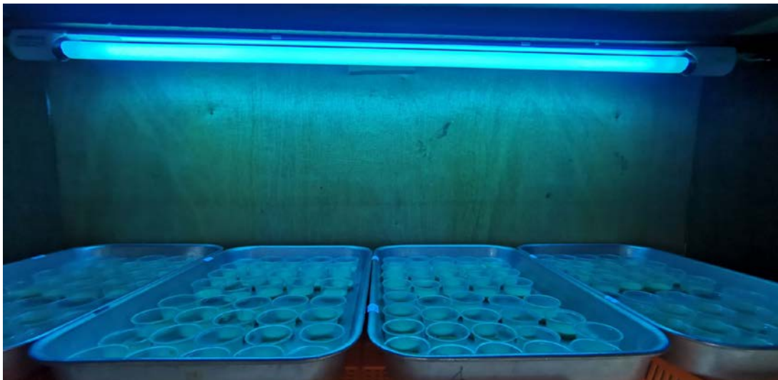
Figure 2 The artificial food coated with SeNPV water-soluble powder to UVB light bulbs exposure
