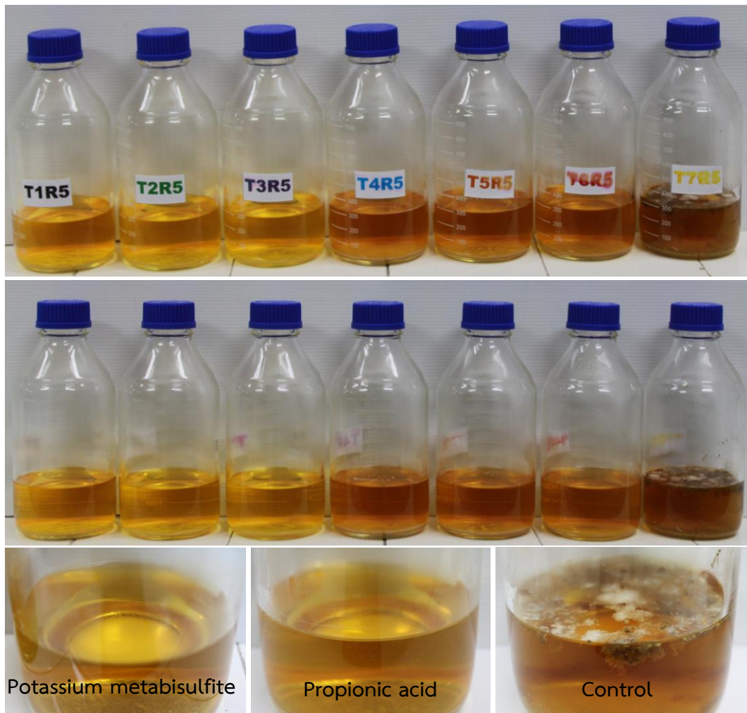
Figure 4 Study on types and levels of preservatives in bioactive compounds from luminescent mushroom “Sirin Rassamee”
