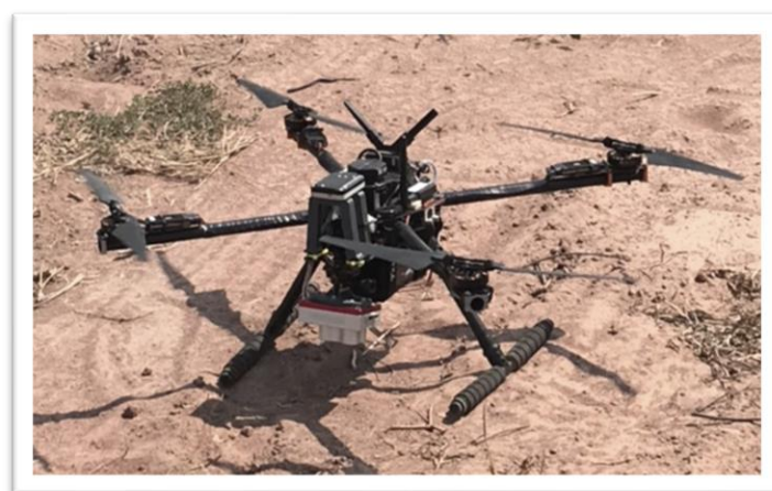
Figure 2 A multispectral imaging camera on Unmanned Aerial Vehicle (UAV) used in this study
