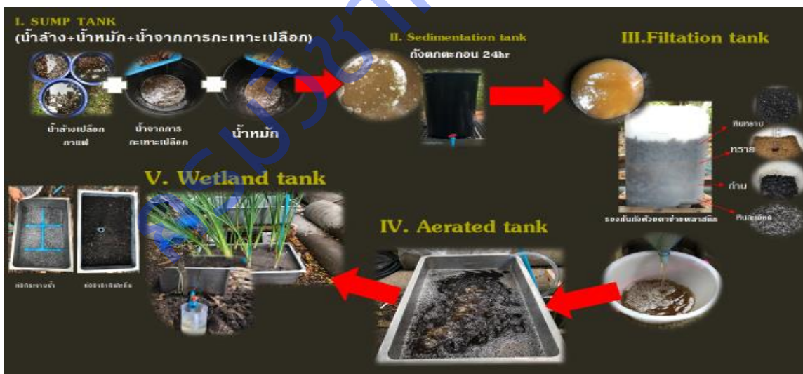
Figure 2 Demonstration protocol of coffee waste treatment method in fifth steps from sump tank to sedimentation tank then the filtration tank combined with aerated tank and stocking the pretreatment water in wetland tank for further used in field or recycling water cycle.
