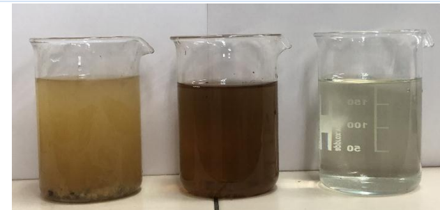
Figure 10 Important following parameter during coffee wastewater treatment important parameter of wastewater during coffee wastewater treatment described in the increasing of water pH contain and the reduction of Total dissolved solid (TDS)
