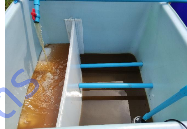
(c) Filtration tank
