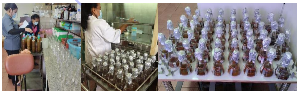
Fig. 10 Ethanol production from juice cane with batch fermentation method using S. cerevisiae
