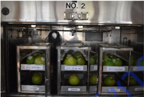
Figure 32 Mortality test of first instar of oriental fruit fly, Bactrocera dorsalis (Hendel) in pummelo Khao Tang Kwa treated with modified vapor heat treatment in preliminary disinfestation test.
