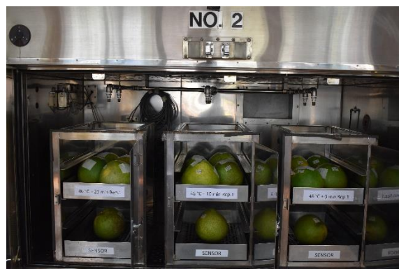
Figure 15. Mortality test of first instar of oriental fruit fly, Bactrocera dorsalis (Hendel) in pummelo Khao Tang Kwa treated with modified vapor heat treatment in preliminary disinfestation test.
