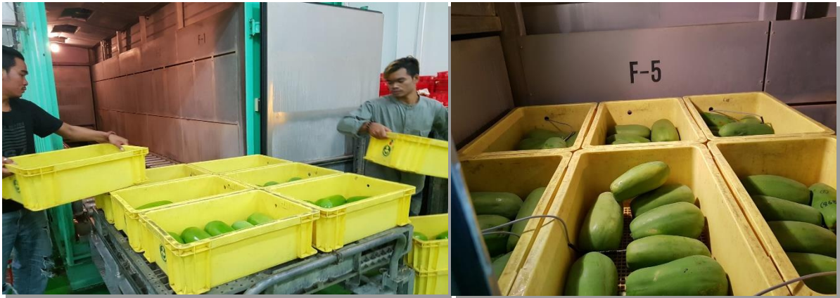
Figure 4 Commercial export simulation test of papaya cv. “Holland” fruit subject to MVHT at 47°C for 20 minutes with full load capacity at Thamai Ariculture Cooperative Ltd. VHT-facility.
