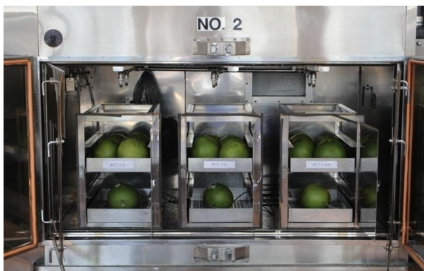
Figure 3 Injury test for Pomelos at Temperature 46 47 48 °C 0 min 1 hr. and 2 hr. of more than 90 % RH for various holding times.
