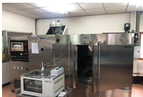
Figure 2 Calibration sensor of resistance thermometers.
