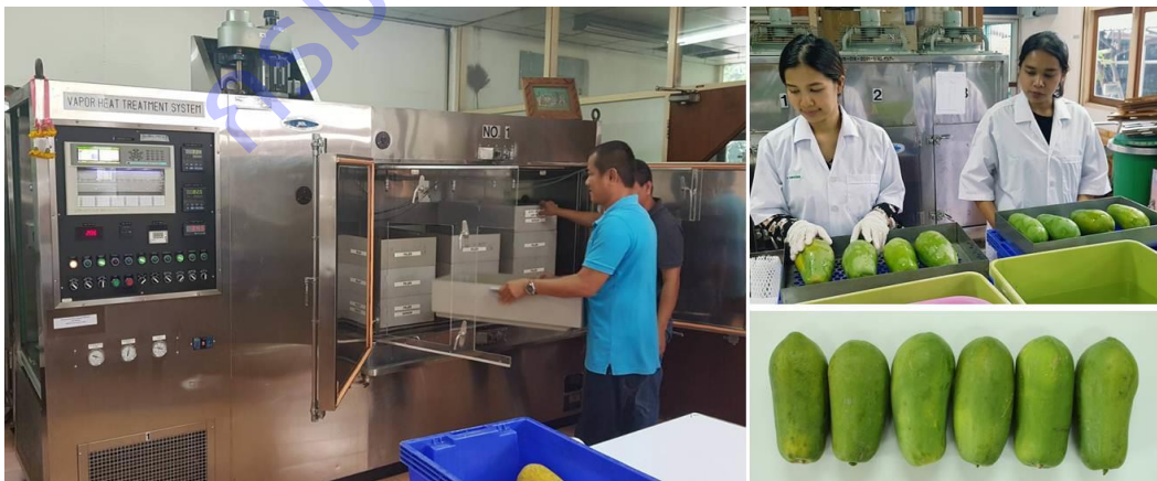
Figure 9 Commercial export simulation test of papaya cv. "Holland" subject to MVHT at 47^{\circ}\text{C} for 20 minutes with full load capacity at laboratory of Plant Quarantine Treatment Section, Plant Quarantine Research Group.
