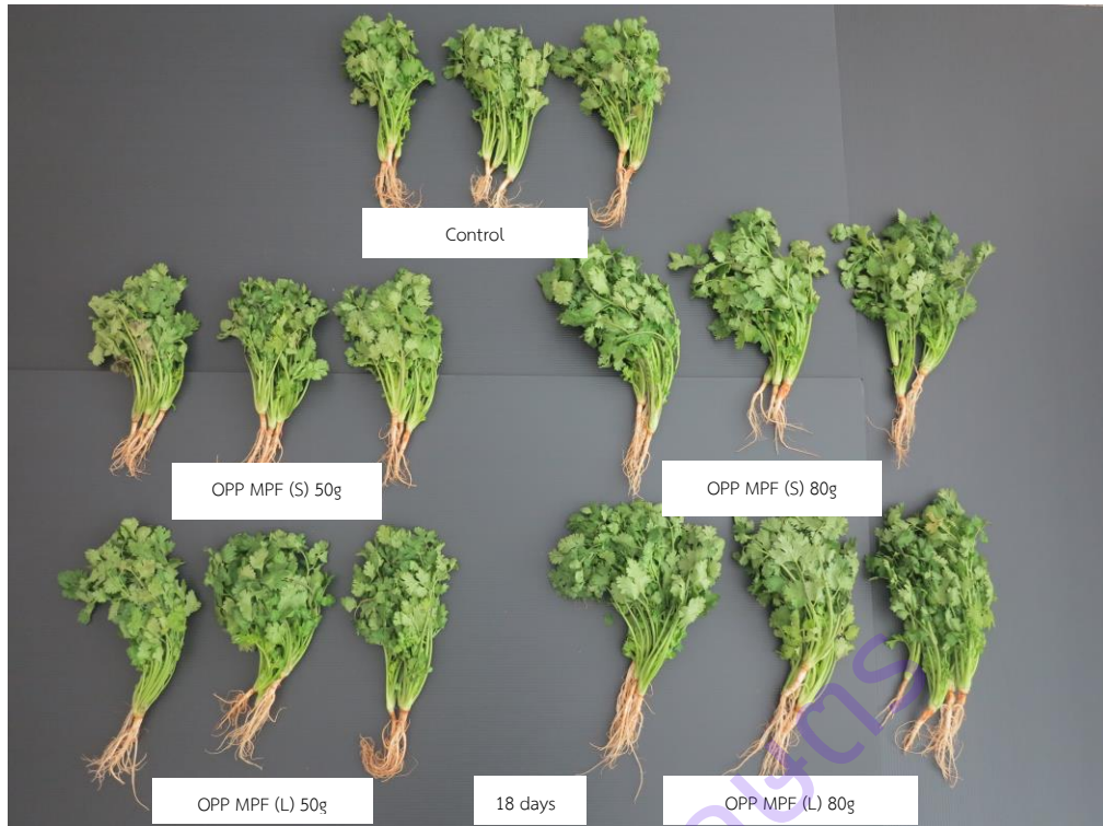
Figure 17 coriander packed in OPP micro perforated film (OTR 5,000-10,000 cm 3 /m 2 /day) storage at 5°C for 18 days
