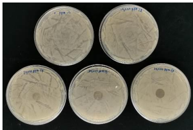
Figure 25 Inhibition zone of PVA films incorporated with various content of dried mangosteen peel powder extract: 0 10,000 30,000 50,000 and 70,000 ppm against Staphylococcus aureus (left to right and top to down).
