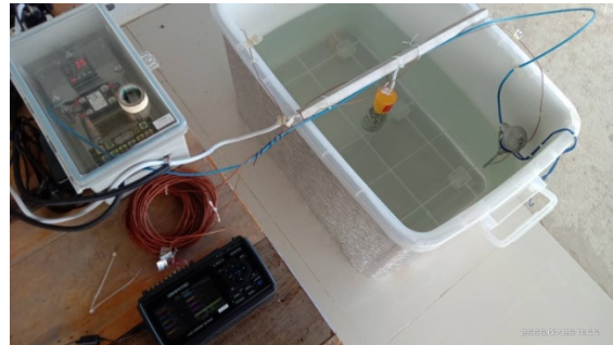
Figure 1 The phototype of virgin coconut oil fermentor consist of Pid temperature control module, 1000 watt heater, type K thermometer and water bin.
