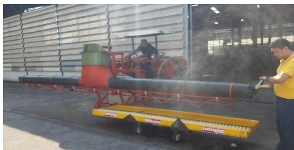
Figure 2 Spraying coverage zone and distance test of nozzle
