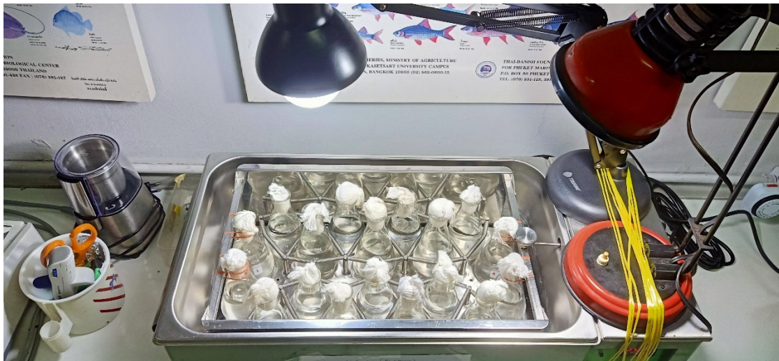
Figure 3 shows the shaking water bath modified for the cultivation of the highly molluscicidal cyanobacteria isolate HMLB05 in BG11 medium on the first day
