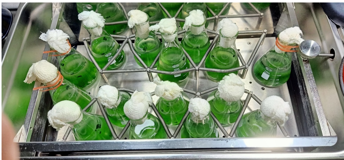
Figure 4 displays the shaking water bath modified for the cultivation of the highly molluscicidal cyanobacteria isolate HMLB05 in BG11 on the 14 th day
