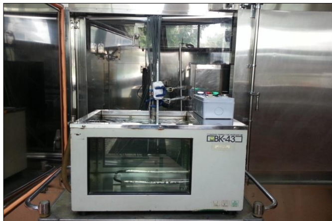
Figure 7 Calibration sensor of resistance thermometers
