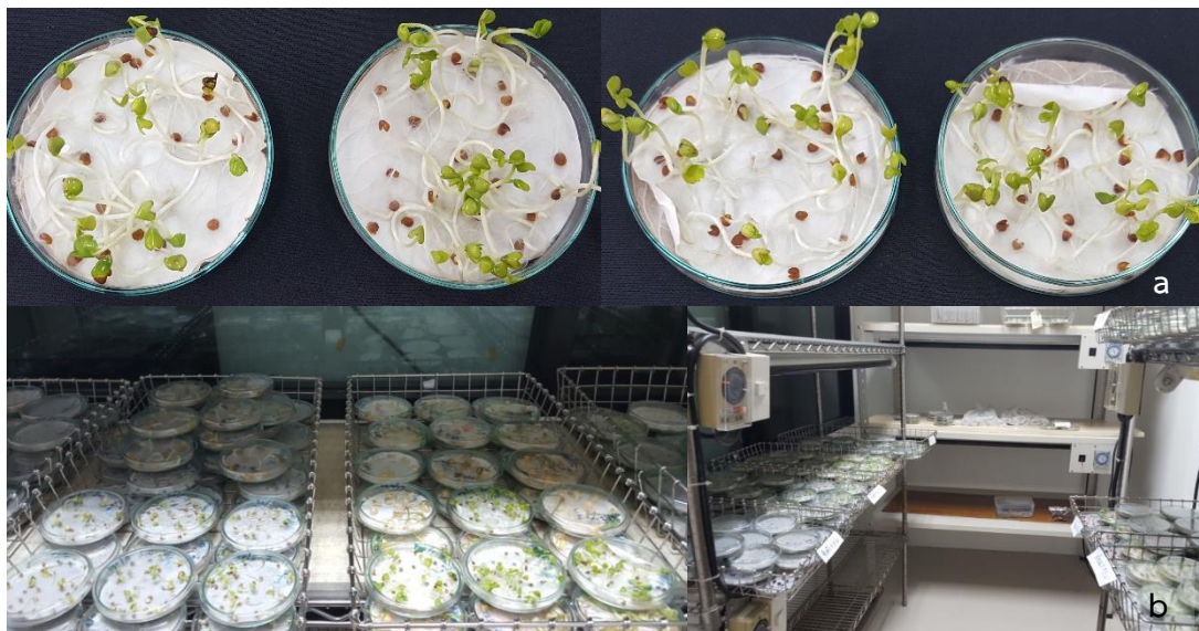
Figure 6 Blotter method. A sample of 400 seeds, 25 seeds in each petri. Incubation facilities: shelve, light arrangements and trays with petri dishes.
