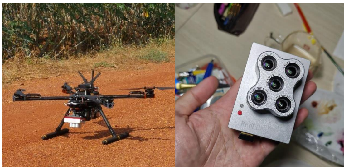
Figure 2 A multispectral imaging camera on Unmanned Aerial Vehicle (UAV) used in this study
