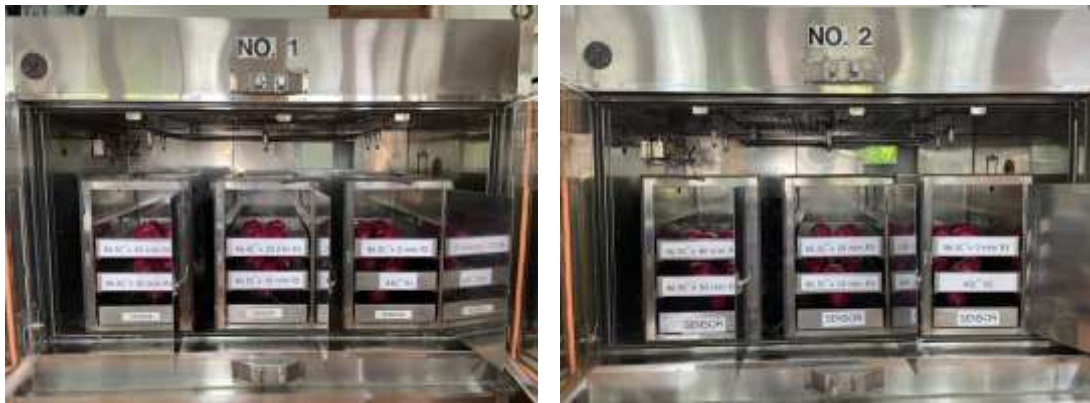
Figure 8 “Sanshu” vapor heat treatment system (differential pressure type) No.1 and No.2 for heat infestation to all stage of Bactrocera dorsalis on red dragon fruit at fruit center temperatures attained 45 and 46.5 c° and kept for 10, 20, 30 and 40 minute
