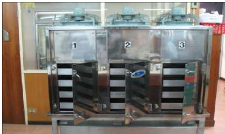
Figure 13 Showing cooling system (differential pressure type) model: SHS-12
