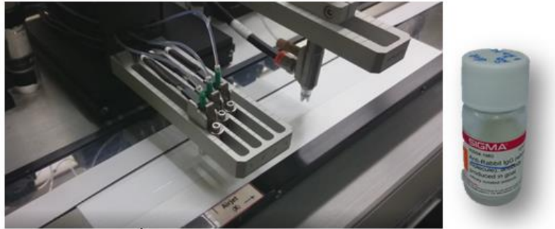
Figure 2 LYSV-IgG spray (concentration 1 mg/ml), volume 1.5 \mu\text{L}/\text{cm} . (test line) and goat anti-rabbit IgG or GAR (SIGMA Co.) spray diluted 1:3 times, volume 1.0 \mu\text{L}/\text{cm} . (control line) with Bio jet spray head
