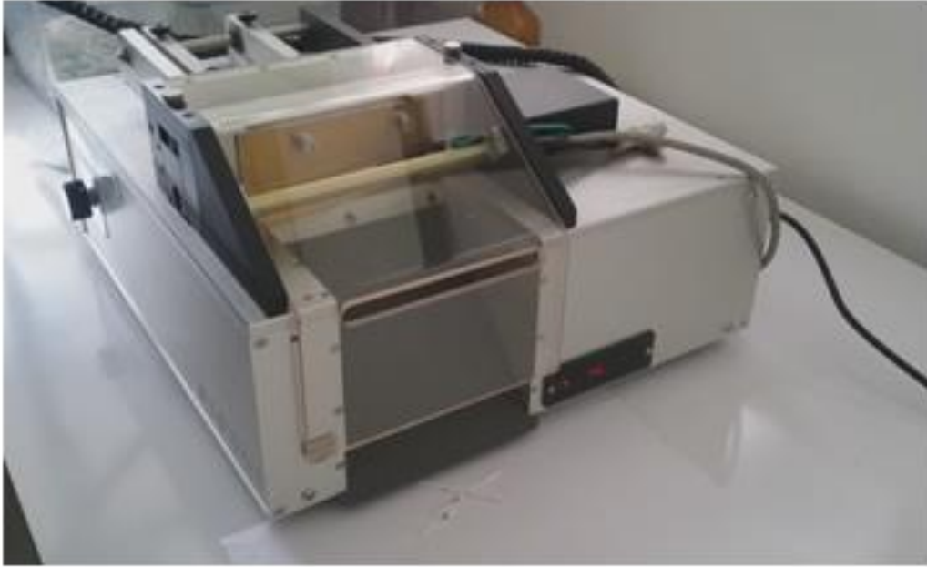
Figure 5 Bio dot automatic cutting machine cuts strips with a width of 0.4 cm
