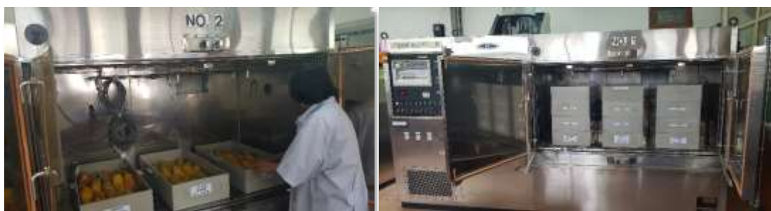
Figure 14 All infested fruits were placed in the containers located in the bottom of VHT chamber (left), large scale confirmatory test was conducted with MVHT at fruit temperature of 47°C for 20 minutes
