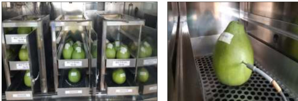
Figure 9 Place monitoring of fruit temperature (sensor fruit).
