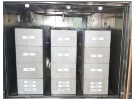
Figure 22 Low load and Full load in chamber (capacity 50 and 100 %)
