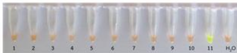
Figure 5 Detection of Pseudomonas fuscovaginae by LAMP. 1-10, rice samples; 11, P. fuscovaginae (positive control); H 2 O, negative control (distilled water)
