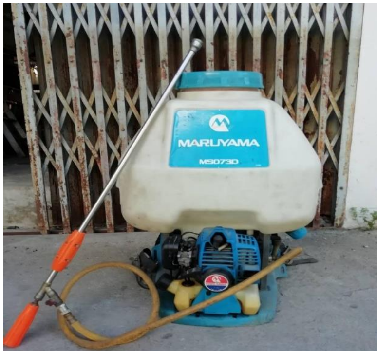
Figure 2 The motorised knapsack sprayer used in the experiments
