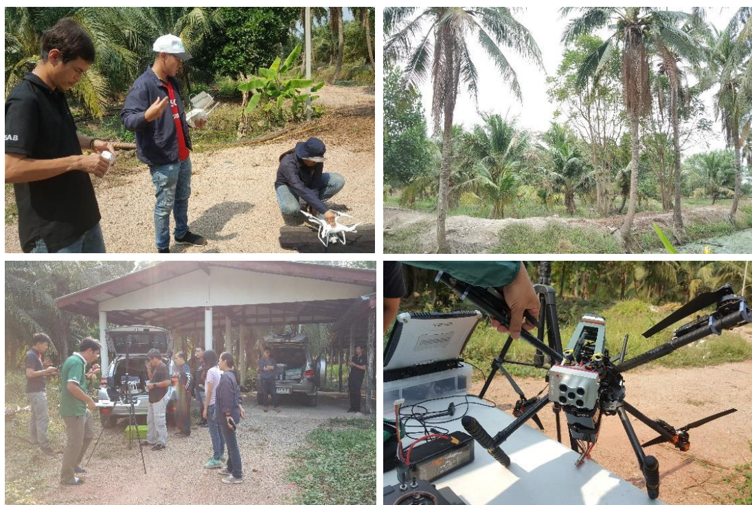
Figure 1 The operation by coconut black-headed caterpillar with a multispectral imaging camera on Unmanned Aerial Vehicle (UAV) in a coconut plantation at Damnoen Saduak district, Ratchaburi province
