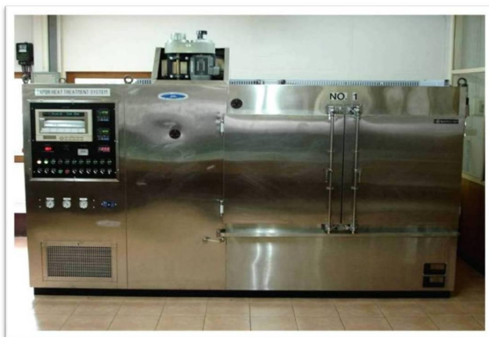
Fig. 1 Sanshu vapor heat treatment system (differential pressure type : model EHK 1000 D) used for experiment of Plant Quarantine Research Group.
