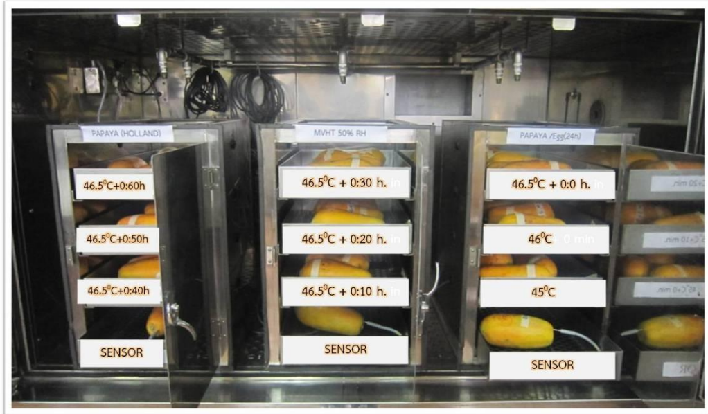
Fig. 6 Susceptibility of stages of B. dorsalis to modified vapor heat treatment test. All infested test fruits were placed in the chamber and monitoring of fruit temperature by using sensors reached the center fruit temperature at 45°C, 46°C, 46.5°C, and maintained at 46.5°C for 0, 0:10, 0:20, 0:30, 0:40, 0:50 and 0:60 h.
