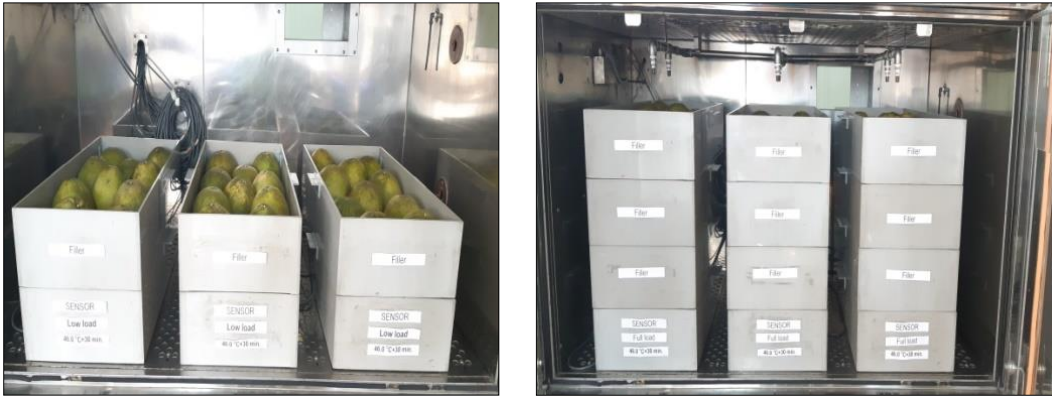
Figure 22 Low load and Full load in chamber (capacity 50 and 100 %)
