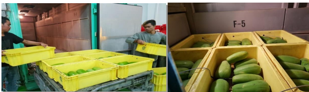
Figure 3 Commercial export simulation test of papaya cv. “Holland” fruit subject to MVHT at 47°C for 20 minutes with full load capacity at Thamai Ariculture Cooperative Ltd. VHT facility.
