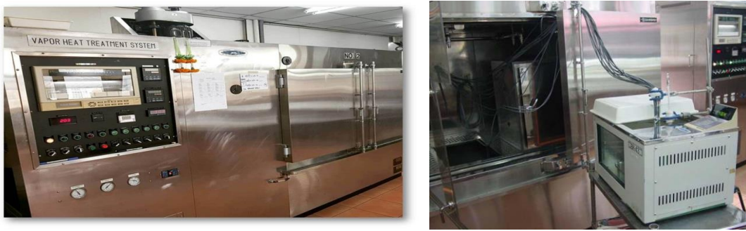
Figure 2 Calibration sensors were conducted by dipping all sensors into constant temperature water bath at 47° C for 20 minutes at laboratory of Plant Quarantine Treatment Section, Plant Quarantine Research Group
