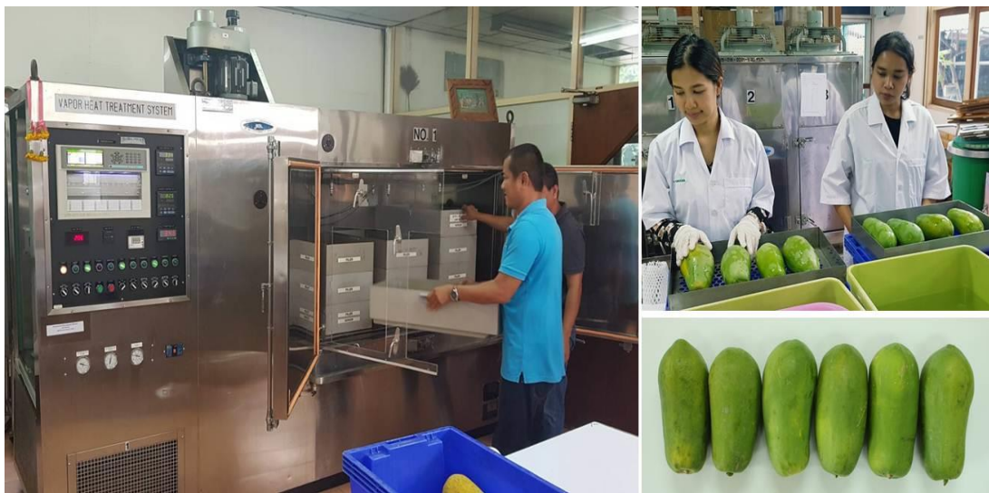
Figure 8 Commercial export simulation test of papaya cv. “Holland” subject to MVHT at 47^{\circ}\text{C} for 20 minutes with full load capacity at laboratory of Plant Quarantine Treatment Section, Plant Quarantine Research Group.
