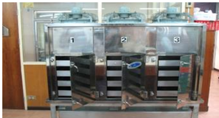
Figure 6 Vapor heat treatment unit and cooling unit: 'Sanshu' Shower Cooling System (Differential Pressure Type), Model: SHS-12
