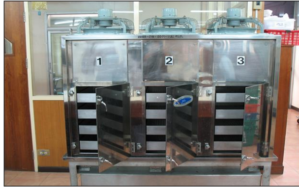
Figure 13 Showing cooling system (differential pressure type) model: SHS-12
