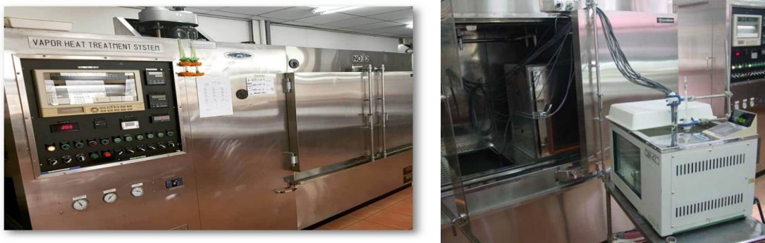
Figure 1 Calibration sensors were conducted by dipping all sensors into constant temperature water bath at 47°C for 20 minutes at laboratory of Plant Quarantine Treatment Section, Plant Quarantine Research Group.
