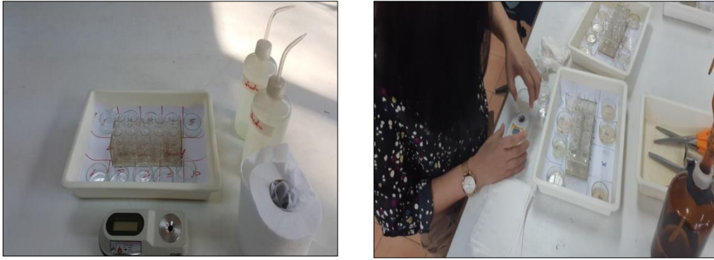
Figure 16 The measurement of total soluble solid (TSS) by using 'atago' digital refractometer (model: DBX-30)
