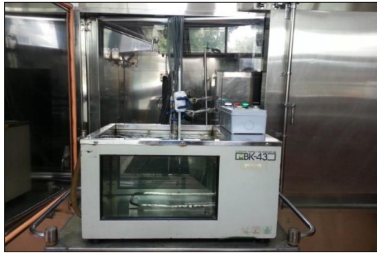
Figure 7 Calibration sensor of resistance thermometers
